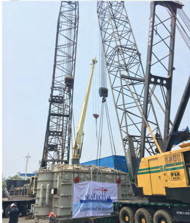
MV MARMOLOKAI, executed shipment for 160 MT Transformer loaded with Shore Cranes at Mumbai Port, to Walvis Bay, Namibia.
